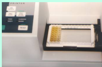
Read plates in a Plate Reader at 450 nm within 30 minutes of the addition of Stop Solution.
