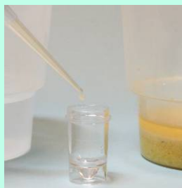
Add Buffer to vial first, then add extract; mix well with pipette tip
