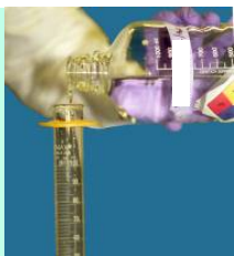
Measure solvent, add to ground sample
