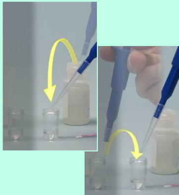
With a new pipette tip, add DB2 Buffer to the second vial (the reaction vial) for testing
