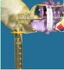
Measure solvent, add to ground sample
