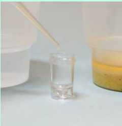
Add DB1 Buffer to vial first, then add centrifuged extract; mix well with pipette tip
