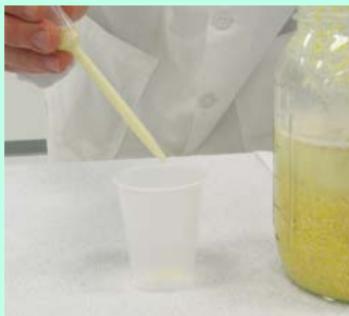
Transfer extract to cup, about 2 pipettefuls
