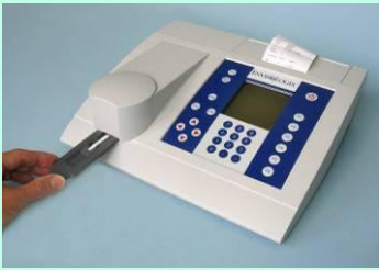
Place QuickStix Strip in holder, insert into QuickStix Reader
