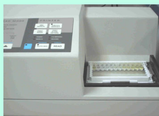
Read plates in a Plate Reader within 30 minutes of the addition of Stop Solution.
