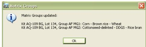
successfully uploaded by matching the Matrix Groups shown on the card to the Matrix Groups shown in the dialog. Once barcodes are uploaded, they will remain permanently in the program’s memory, and thus the card will not need to be scanned again. Please note: the Barcode Card will need to be scanned each time you receive a new lot of strips.
