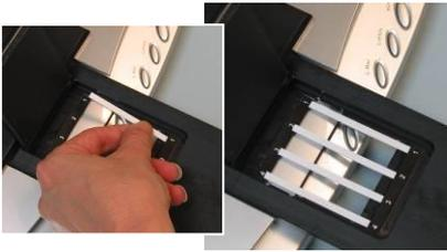
When reading single strips, up to four individually barcoded tests can be read at one time. Proper spacing is important, so numbered positions have been etched into the carrier. Load the strips using the step-by-step instructions above, carefully placing them in the desired positions. Place the first strip in Position
