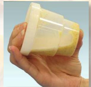
3. Shake 1 minute on mechanical shaker or by hand for 1½ - 2 minutes
