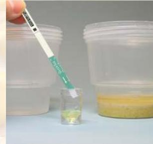
6. Stir well with pipette, then add test strip; wait 5 minutes for results
