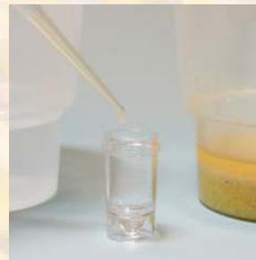
5. Add 100 µL Buffer to vial, then using a new pipette tip, add 100 µL sample to vial
