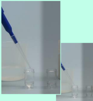
Add 50% ethanol then the sample extract to the first vial (the dilution vial) and mix. Discard pipette tip.
