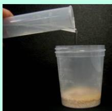
Measure Grain Buffer, add to ground sample
