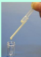
Transfer of clarified extract to a reaction vial using a fixed volume transfer pipette
