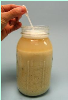
Avoid pulling up particles when drawing sample
