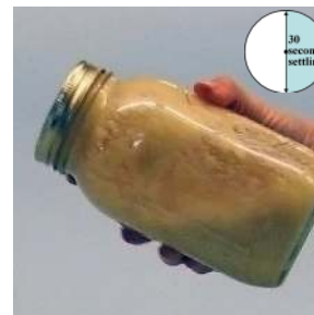
2. Shake vigorously for 30 seconds, then settle 30 seconds
