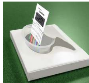
5. Insert comb into cup with arrows pointing down; wait 5 minutes
