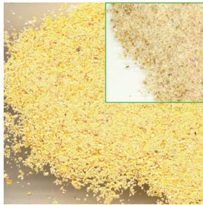
1. Collect and grind representative sample such that  $\geq 95\%$  passes through a 20 mesh sieve
