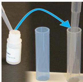
7. Using a new tip, add 100  $\mu$ L Buffer to the clear testing tube
