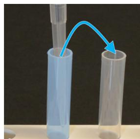
8. Transfer 100  $\mu$ L of Step 5's diluted extract from the dilution vessel to the clear tube; stir well with pipette tip
