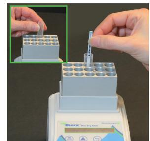
9. Place clear tube in Incubator and acclimate for 2 min.\*, then add QuickTox Strip; wait 2 minutes for results
