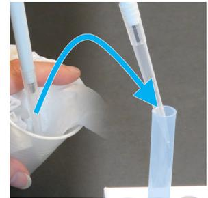
5. In a separate vessel, dilute extract with water\* 1:8, for example, 100  $\mu$ L sample extract to 700  $\mu$ L water (measure carefully!)
