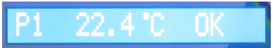
Run all Flex assays in the incubator. If the temperature of your room is between 20 and 24°C (68 and 75°F) you may skip the 2 minute sample acclimatization step. Set the test tubes in the incubator, extract your sample, transfer extract to the tube along with buffer, and run the test in the incubator.
