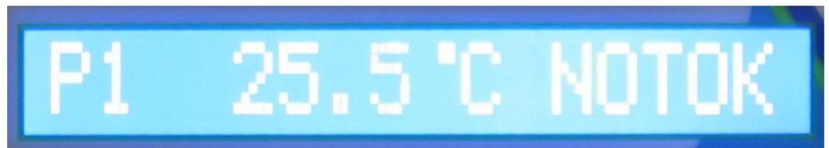
Once the correct temperature is within range, it will beep and the readout will change to "OK".
