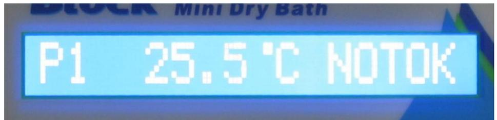
Once the correct temperature is within range, it will beep and the readout will change to "OK".
