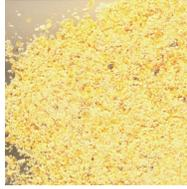
1. Collect and grind a representative sample such that  $\geq 95\%$  passes through a 20 mesh sieve
