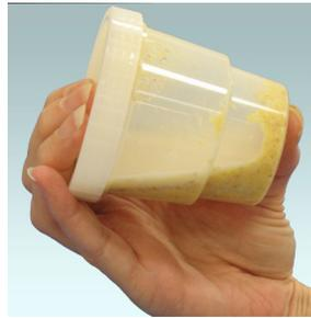
3. Shake 1 minute on mechanical shaker (>300 rpm) or vigorously by hand for 2 minutes
