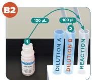
Using a clean tip, pipette 100  $\mu$ L of **DB5** into a clear **Reaction Tube**, then transfer 100  $\mu$ L of diluted extract from the blue **Dilution B Tube** and mix well.
