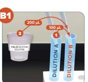
In a clean blue **Dilution Tube**, mix 100  $\mu$ L of **Diluted Extract** (saved from step A1 above) with 200  $\mu$ L of **Dilution Solution** and mix well.
