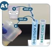
In a blue **Dilution Tube**, dilute 100  $\mu$ L of clarified extract with 400  $\mu$ L of **Dilution Solution** and mix well.
