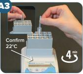
Place **Reaction Tube** in the Incubator for 2 minutes.\* Add a new test strip - arrow tape down - and allow to develop for **4 minutes**. Select **Dilution 1:A** on your QuickScan results screen.
