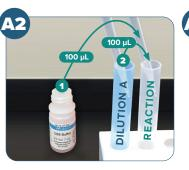
Using a clean tip, pipette 100  $\mu$ L of **DB5** into a clear **Reaction Tube**, then transfer 100  $\mu$ L of diluted extract from the blue **Dilution Tube** and mix well.
