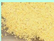
Correct 20 mesh grind for corn
