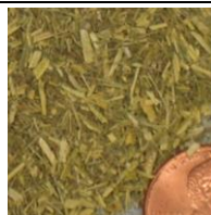
Ground for 1 minute, contains plenty of 40-mesh particles—test the finest particles possible
