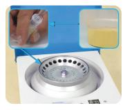
Centrifuge a portion of extract for 30 seconds at 2000 x g (NOT RPM).
