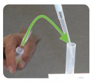
7 Transfer 100 μL of the clarified extract to the tube; stir well with pipette tip
