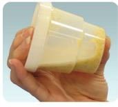
Shake for 1 minute on mechanical shaker (or vigorously by hand for 2 minutes)
